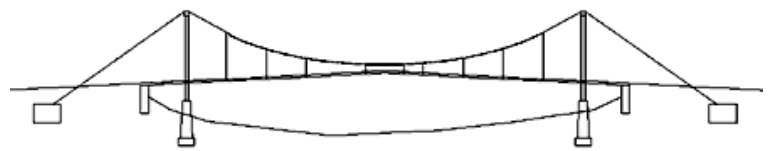
Cable suspension bridge without stiffening truss
